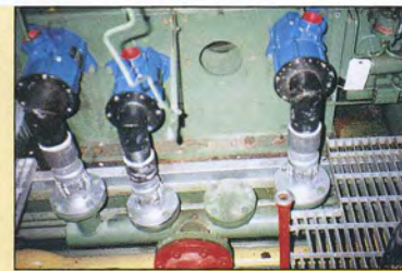
A trio of T100-Ds on a Clark gas engine provide the reliability to handle the higher cranking speeds.
